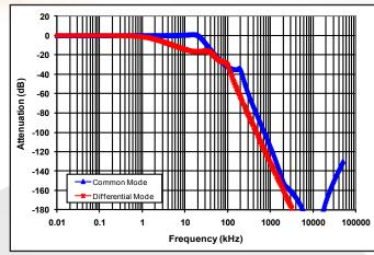
Figure 1: Typical Common Mode and Differential Mode Attenuation provided by the filter as a function of frequency. Both input lines are connected to chassis ground through  $50\Omega$ resistors. The filter case is also connected to chassis ground.
